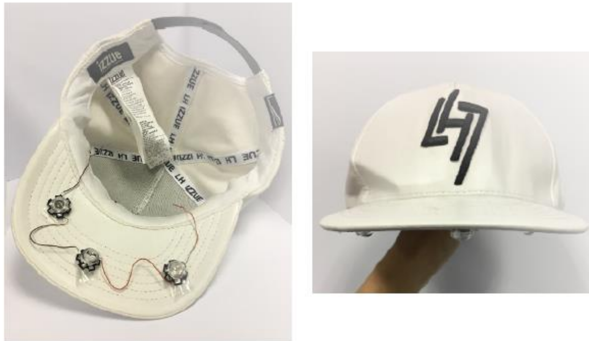
Figure 4.4: Physical-world infrared adversarial device from [103].
