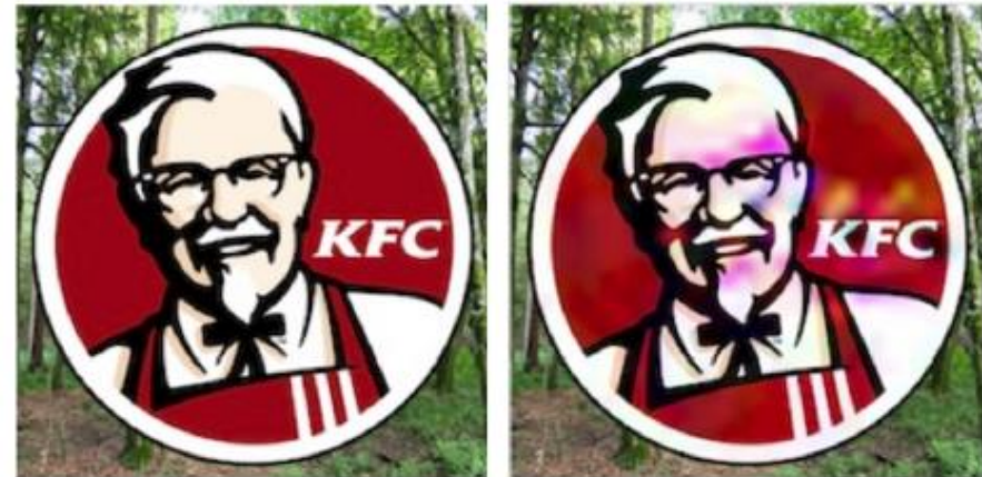
Figure 4.3: Clean advertising sign (left), reasonably rejected by the traffic sign recognition system, and its adversarial counterpart (right), recognized as a "stop" road sign, from [101].
